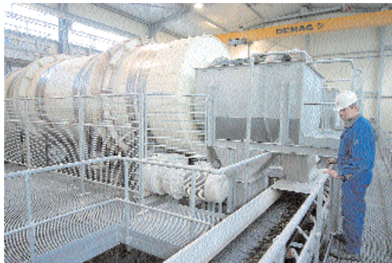
Fig. 1 Amberger Kaolinwerke: Suspension of valuable crude ore in water in first coarse separation stage for mineral components kaolin, feldspar, and quartz sand
